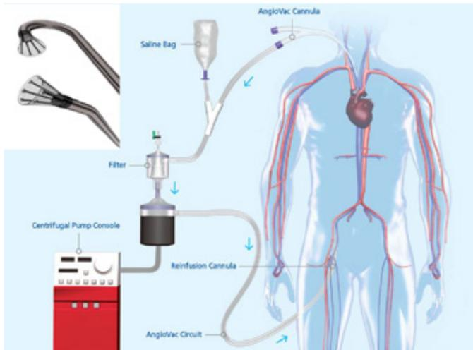
**Figure 1.** The AngioVac system and its associated 20° and 180° funnel-shaped cannulae. Arrows indicate the flow of blood from the inflow AngioVac cannula in the IJV through the thrombus filter, centrifugal pump and AngioVac circuit to venous return via femoral vein. Reproduced with permission from AngioDynamics.
